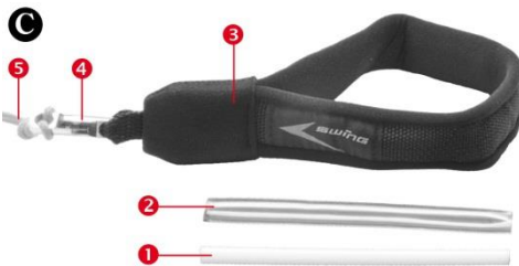
Multigrip brake handle after removing both stiffening rods. These are the various parts:
